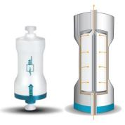
Figure 2: CIMmultus™ 8 mL Advanced Composite Column (left) operates with unique 'radial flow' direction (right) whereby solutes enter the stationary phase across the length of the tubular monolith; separation takes place across the width of the tube wall.
